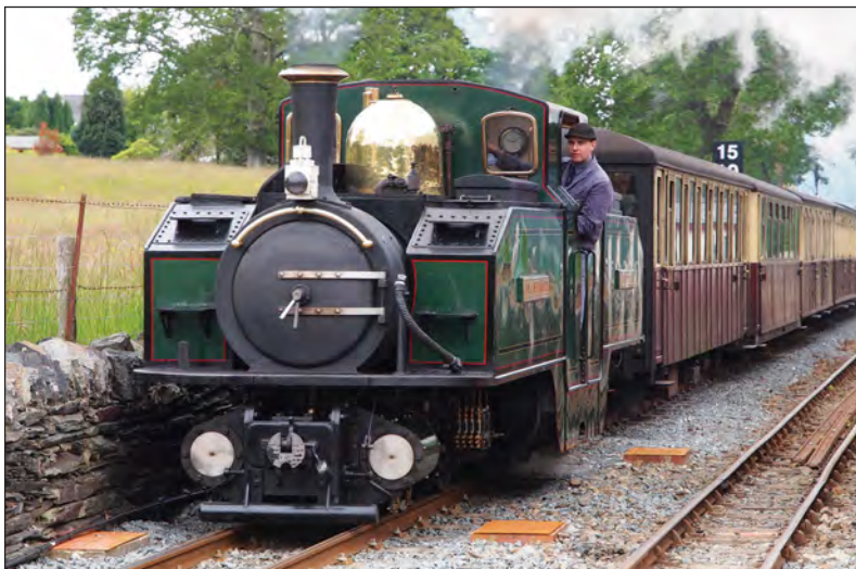
Above: The Earl passes Boston Lodge works on its first run after being converted to coal firing, on 5th July 2006.
